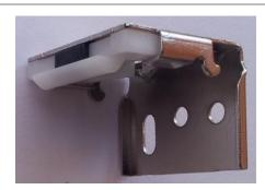
1. Position the end brackets for fixing (either Inside Mount or Outside Mount) ensuring that the brackets are fixed approximately 50mm from the end of the blind. The centre bracket (required for blinds exceeding 1200mm width) may be positioned as required.
