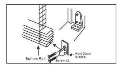
The use of hold down brackets is recommended for additional child safety, but is not a requirement for the normal functioning of the blind. Using the two screws provided, attach the base of the hold down bracket to the window facing or sill. Additional fixing can also be fitted through the side of the bracket (where suitable). Snap bracket pin ends into the holes in the ends of the bottom rail.
