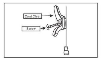
Cord cleats must be installed to comply with Regulations. The cleats must be installed at least 1600mm above floor level, because a child is capable of unwinding a cord from a cleat. Fasten the cleats to the wall using the screws provided. Do not use tape or glue to attach the cleats.
